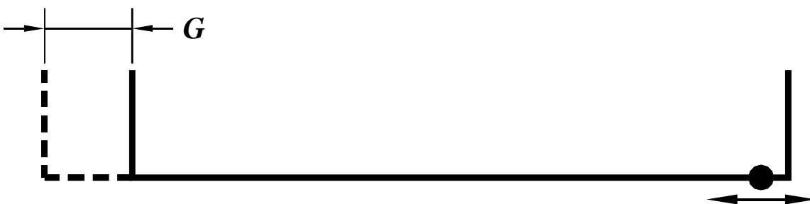
Figure 2. Hot Piping Run with One Longitudinal Restraint at the End of the Run
